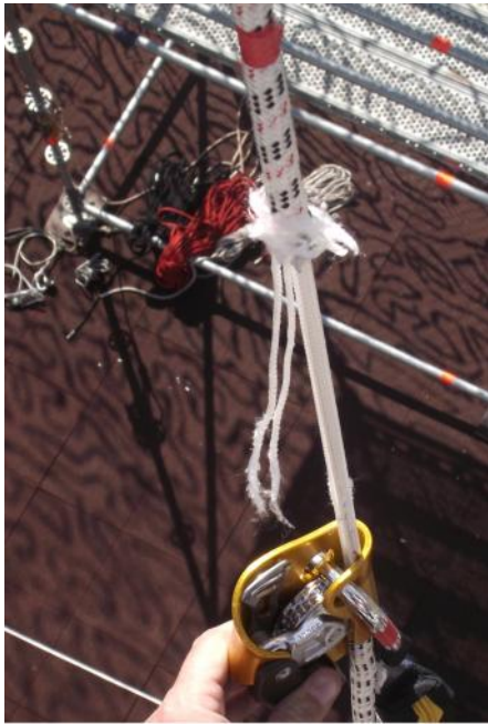
Damage – 1 st ASAP 100kg Drop Test
