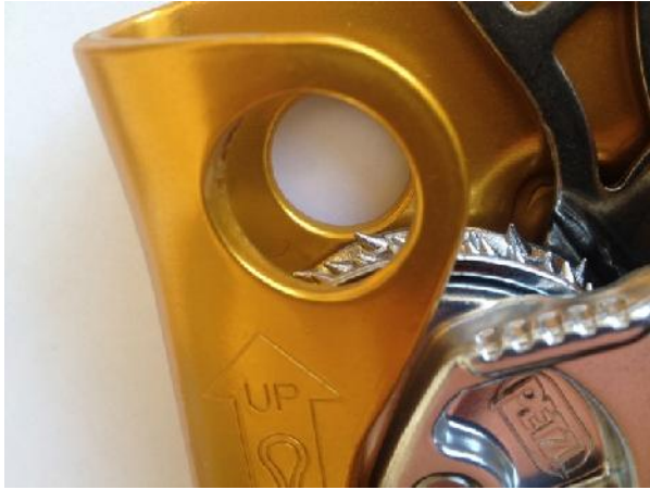
New – No damage to body at clip point.
