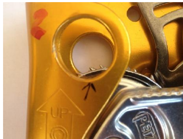
Damage after 100kg Drop test – section of 'wheel' visible
