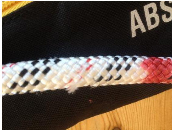
2 nd 100kg Drop Test. Minor damage to rope caused by teeth. Red mark indicates stopping position of the top edge of the ASAP.
