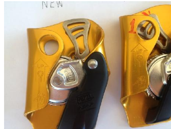
Deformation caused by Karabiner during 100gk drop test.
