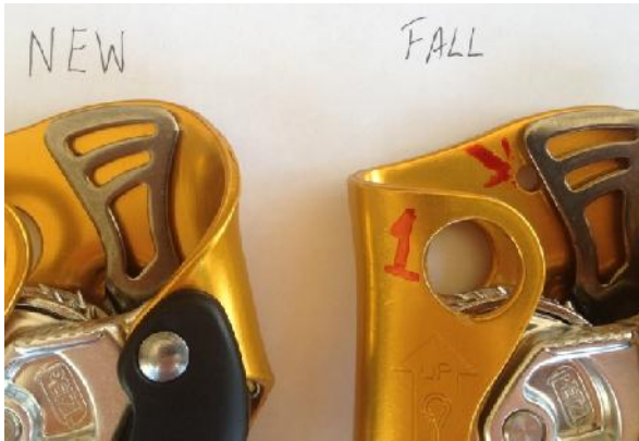
Deformation of device – small hole at top of device exposed.
