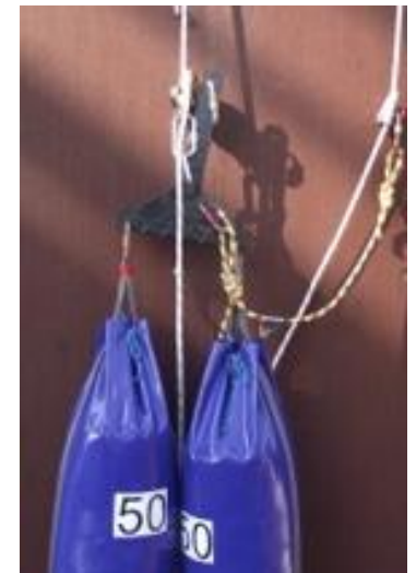
Pictures showing the test plate with both waist and chest attachment points.
