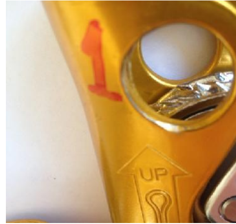
Deformation caused by Karabiner during 100gk drop test.
